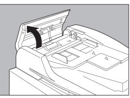
**2** Open the Inner Cover while holding the green-labeled tab.
