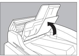
**4** Open the Exit Guide while holding the green-labeled tab.
